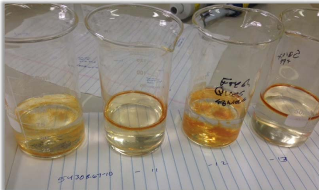
Figure 6. Several tested conditions of iron addition for recovery of entrained extractant.
